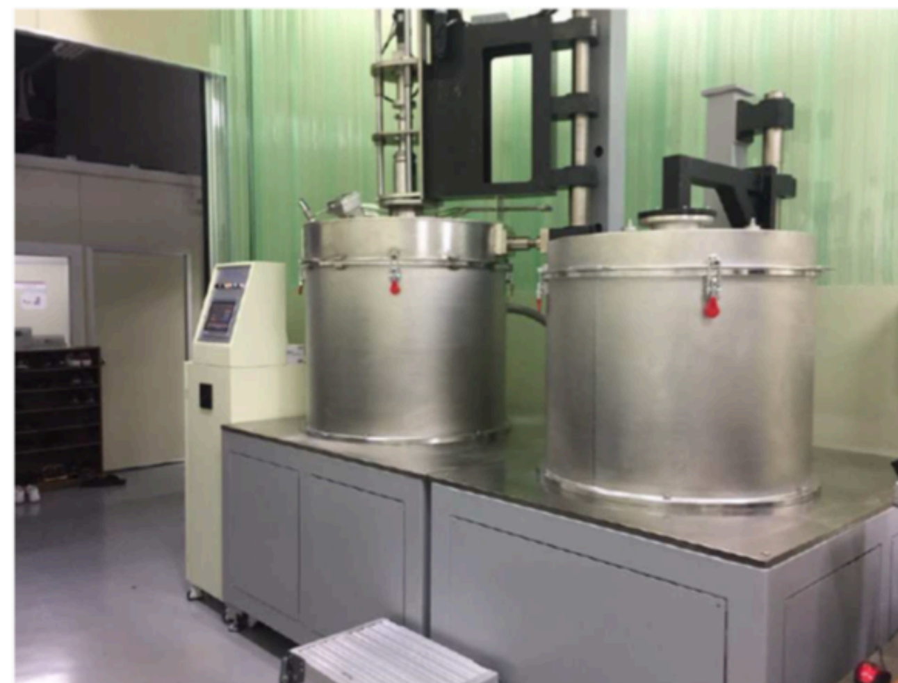
~ 100 kg NaI crystal (ingot) grower
