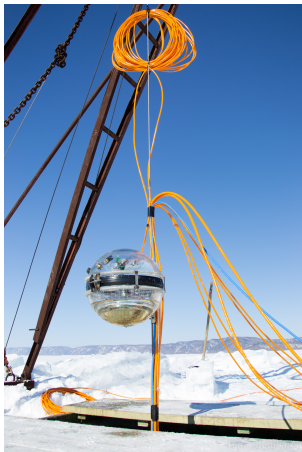
Optical Module (OM) PMT: Hamamatsu R7081-100
