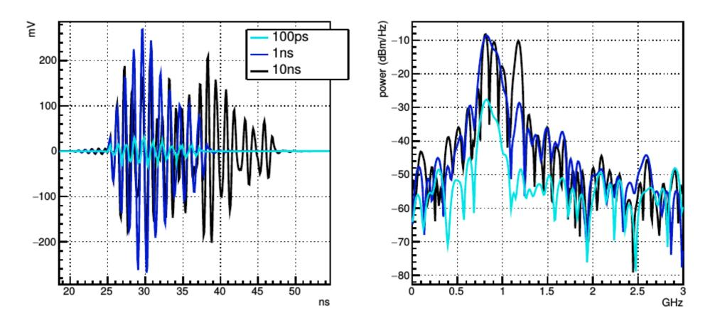
signals vary based on the free electron (plasma) lifetime.
