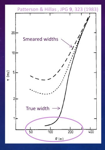
At sufficiently high energies, larger detector spacings can be used to measure the time-width at a given *R*.
