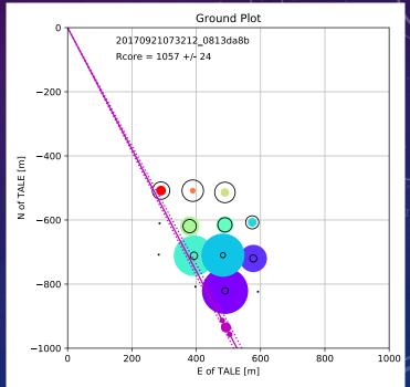
NICHE counter locations, signal size (filled circles), relative time (color) and width (open circles). Intersection of TALE SDP with ground shown and core position shown in purple.
