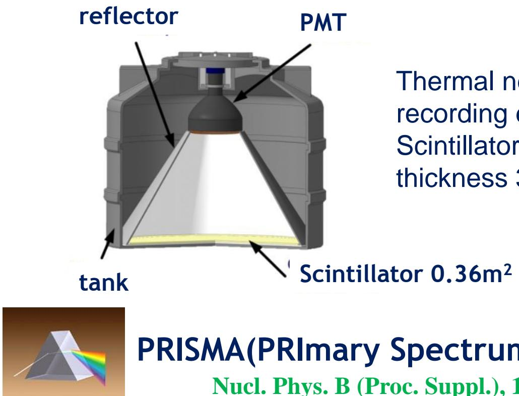
Thermal neutron recording efficiency ~20%. Scintillator effective thickness 30 mg/cm<sup>2</sup>.
