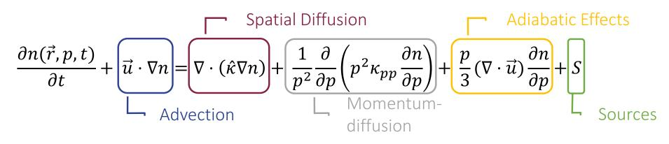
Partial (Fokker-Planck) Differential Equation (FPG) for particle density n
